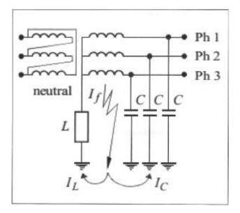
Here are grounding connections on the secondary side of the power transformer coming into a structure. The illustration is for 3-phase (Single phase is the same grounding scheme). Here is shown an inductive element (L) in series with the Y-Connected secondary's common ground and also has three capacitive elements across the phases to ground in order to provide an additional safety path without costing too much energy budget.
