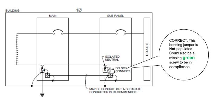
Notice there are two panels shown here; the **main** panel has the Neutral bonding lug connected to the Equipment grounding lug with what's known as a jumper while ..... (IMPORTANT!) the **sub-panel** downstream has that jumper removed.
