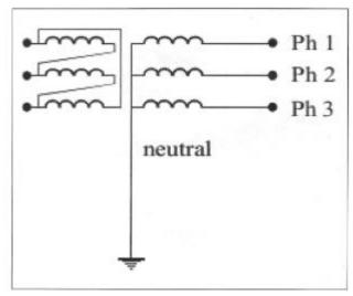
Here are grounding connections on the secondary side of the power transformer coming into a structure. 3-Phase Y-Connected in this approach:
