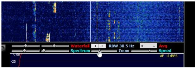
3. Using your mouse wheel you can find tune the radio if you clicked on a frequency and weren't quite on the right spot. I have mine configure to change the frequency by .1 Mhz which generally is responsive enough. Those options are shown here.
