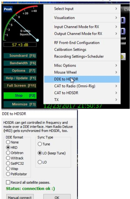
8. After selecting HRD on the above screen, click on manual connect, and the connection should show up as status ok. If it doesn't connect, make sure HRD is on, and communicating with the rig. Try it again.
