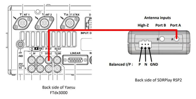
Connect the IF out to the Antenna A of the SDRPlay radio, you will need to use an RCA to a SMA Male cable. I made one of these cables just make sure the SMA is a male connector with a pin in the center. HRO does have crimp style SMA, I solder the center pin and crimped the shield sleeve fairly easy. I purchased PuleLarsen SMA-CP58 from HRO. You can get a premade 3 foot RCA to SMA cable as well, look for ABR Industries 218XATC-SM-RCA-3 from HRO.
