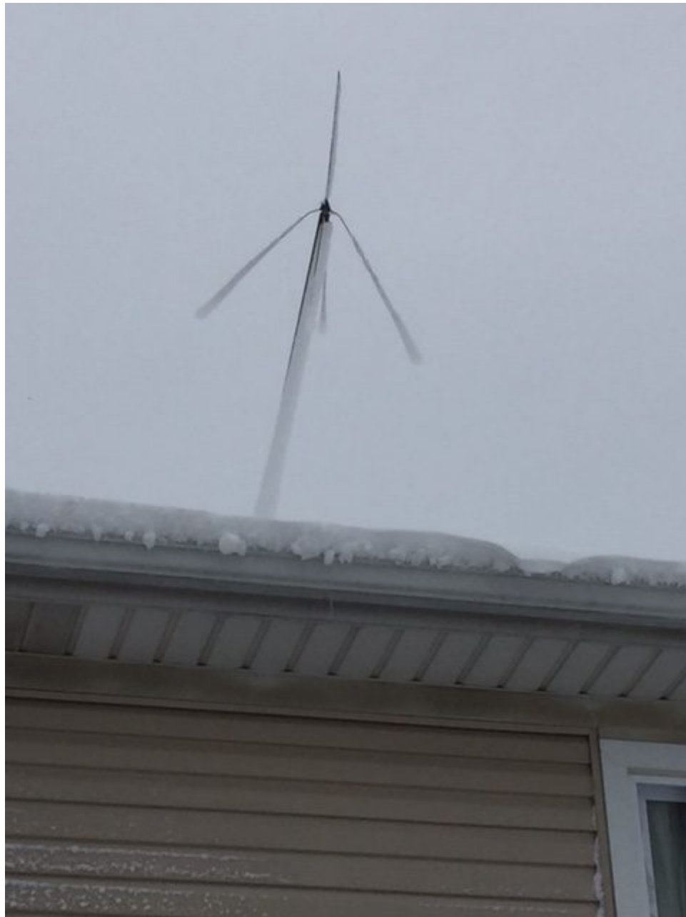
KC9SGV found a lot of ice on a roof-mounted vertical.
