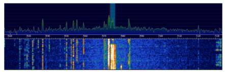
**Dipole Receive** – Below is a screen shot of the panadapter, you can see that the receive is has a flat response across the entire band (click image to expand).
