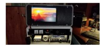
Next, I wanted the ability to run either off batteries or 120v, so I add at Samlex battery backup module(BBM-1225) This neat little device will charge a 12v lead acid battery from the Samlex 12v power supply. If the power supply is off, the battery will take over without any cable changes.
