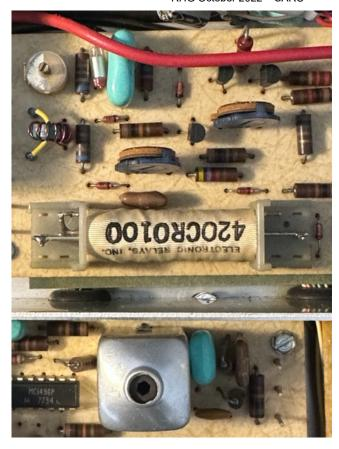
Upon opening the radio this morning in preparation for the repair, I ran a few resistance tests and found the issue! The common lead on the relay was tack-soldered to the carrier board pin. The solder connection had fractured and the wire was sitting loosely against the pin. 2 seconds with a hot soldering iron fixed it!
