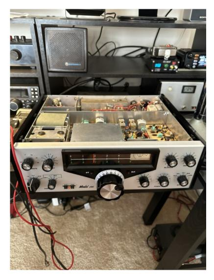
This is a common issue, but the relays with correct form factor are hard to locate. The repair wisdom is to replace the tiny glass-encapsulated magnetic reed switch inside the coil. I located and ordered the needed switches on Amazon.
